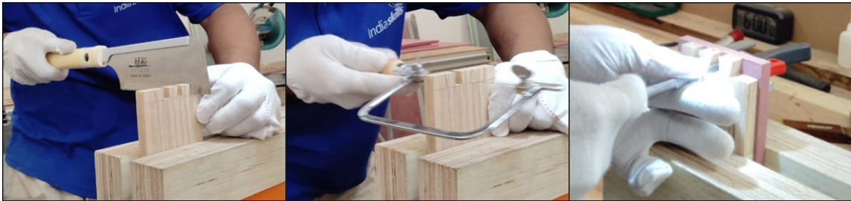
Use dovetail hand saw for cutting tails & pins
