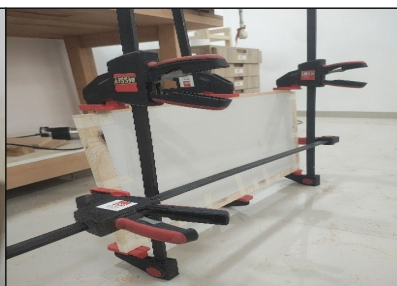
Use F-clamp for fixing top panel bidding
