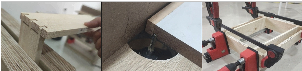
Use router machine for 7.5mm grooving the side panel of drawer box
