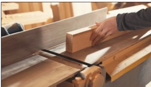
Surface planning at 90-degree angle
