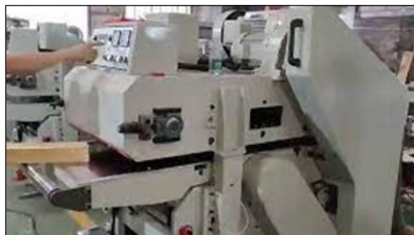
Thickness planning in accurate required size
