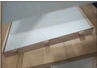
Check domino drill by using dowel
