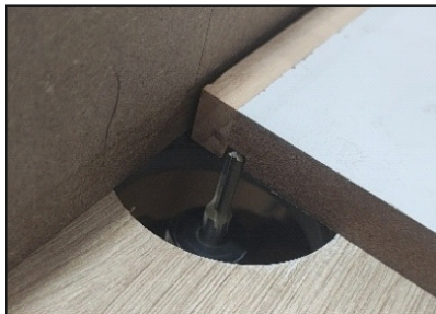
Use 7.5 mm grooving router bit for groove
